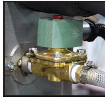
Optional Make-up solenoid valve Figure 3.2A
