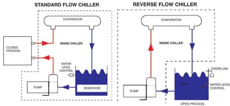
Note - items shown within the dotted borders represent components located inside the chiller.
