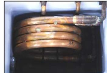
Typical tube-in-tube evaporator shown inside reservoir.
